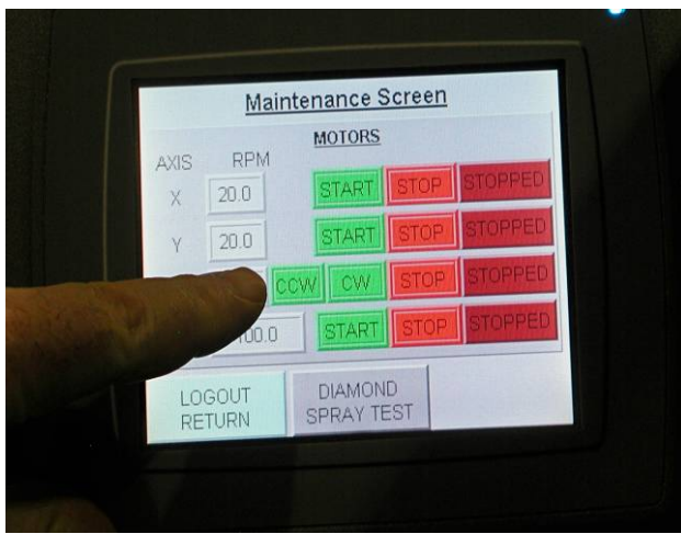
Manual Process Screen (also called 'maintenance screen')
