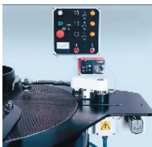
Yoke for workholder ring showing positive drive to roller bar bearing, and reciprocating drive housed below work table surface.
